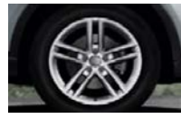
C3P - Audi Exclusive cast aluminium alloy wheels, 5 twin-spoke design, size 7 J x 18, with 235/50 R18 tyres
