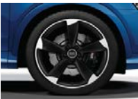
F13 - Cast aluminium wheels in 5-arm rotor design in matt black, high-gloss turned finish. Size 8.5J x 20 with 255/35 R 20 tyres
