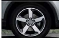
C3I - Cast aluminium alloy wheels, 5-arm design, size 7 J x 18, with 235/50 R18 tyres
