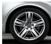
Cast aluminium wheels in 5-arm structured design. Size 7.5 J x 18 with 225/40 R 18 tyres (CS1)
