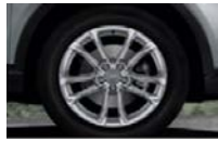
C2I - Cast aluminium alloy wheels, 5 twin-spoke design, size 7 J x 18, with 235/50 R18 tyres
